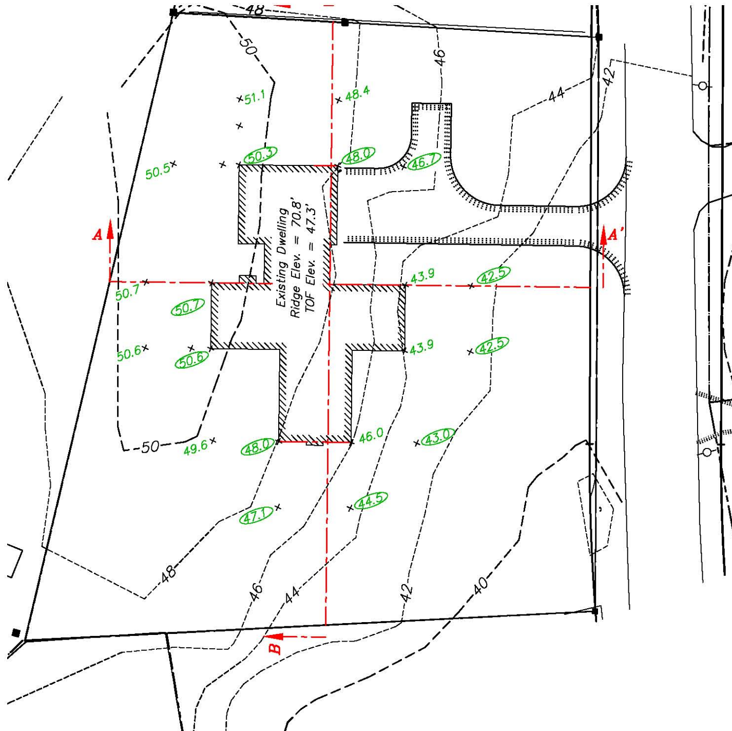
Existing Undisturbed Grade
