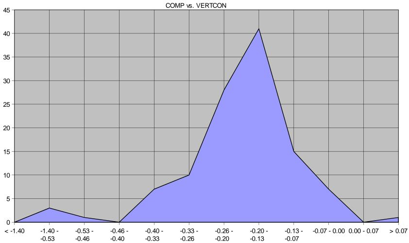
Distribution of the difference between COMP (the comparison of the published benchmark elevations) with the difference determined by VERTCON at the location of the benchmark.
