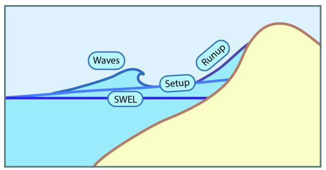
**Figure 2.** The coastal storm surge stillwater elevation (i.e., the line labeled SWEL on the figure) and the added effects of wave setup and wave runup. Figure modified from FEMA Region II Coastal Analysis and Mapping website (www.region2coastal.com/coastal-mapping-basics).
