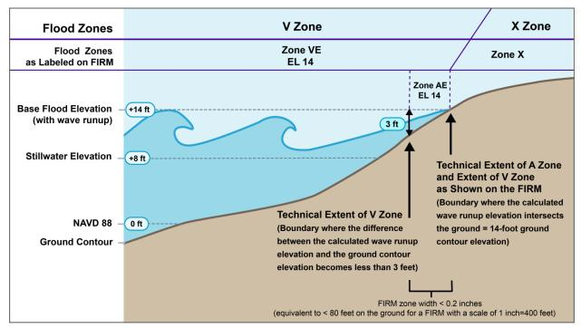
**Figure 5.** Cross-sectional diagram of flood zones on a steep embankment with runup. Here, an A Zone is shown in the profile, but would not be mapped on the FIRM because the zone is less than 0.2 inches in width on the FIRM—thereby not meeting the minimum zone width for mapping at the scale used for FIRMs. Where A Zones such as these are not mapped, the V Zone will extend to the designated ground elevation that corresponds to the V Zone BFE on the FIRM.
