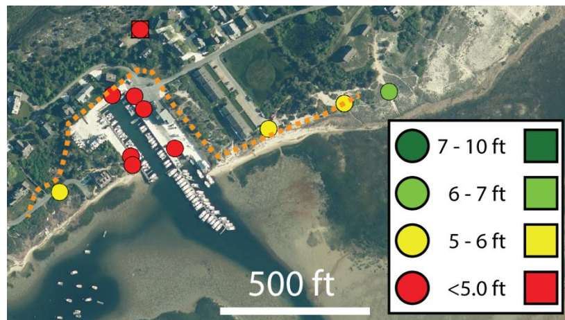
Figure 4. The orange line represents an area that could be addressed to reduce or eliminate storm tide flooding for a significant area of Little Beach lying below elevation 5 ft NAVD88 that experiences inundation from the Atlantic Ocean. All elevations are in feet and refer to NAVD88.
